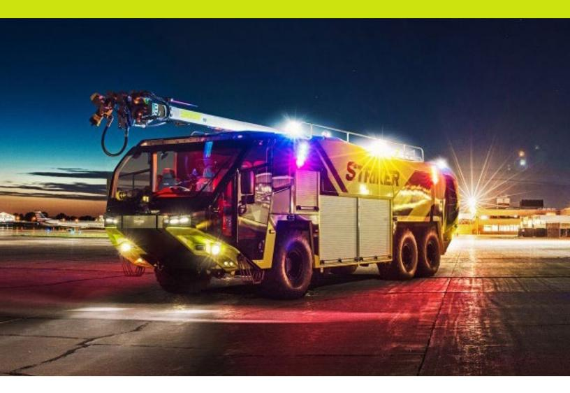
Most ARFF vehicles feature a slanted body with front bumper designed for maneuvering through ditches and rough terrain. Because ARFF vehicles do not need to navigate the confines of a city street, the apparatus is larger than municipal fire trucks. This allows them space to carry more water, necessary gear and equipment, and up to five personnel.
